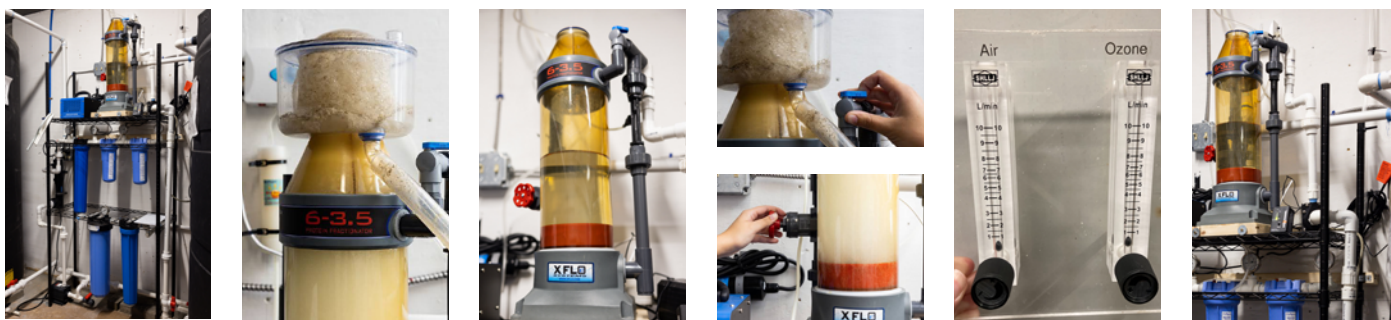
From left to right: Positioning, waste collection, adjustments, top: water input volume, bottom: output valve, ozone/aeration control, and pump compatibility
